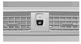
Pressing the button for the central locking system locks and unlocks the doors and the trunk lid when the front doors are closed, but they are not secured against theft.
