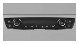
If the drive is continued within approx. 15 minutes, the seat heating is activated automatically with the temperature selected last.
