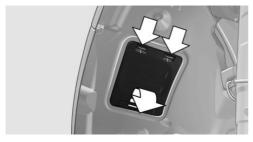
If necessary, pull the inside trim of the wheel house slightly inward. Turn the bulb holder counterclockwise and remove.
