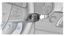
Press the button on the wiper lever.
