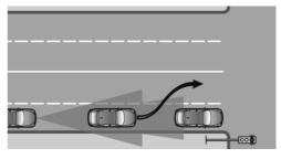
If a vehicle ahead of you unexpectedly moves into another lane from behind a stopped vehicle, you yourself must react, as the system does not react to stopped vehicles.
