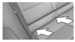
Mounts for the lower LATCH anchors are located behind the indicated covers.
