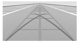
Turn the steering wheel to the point where the pathway line covers the corresponding turning circle line.
