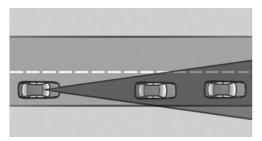
Vehicles are observed when they are traveling in the same direction of movement if they are located within the detection range of the system.
