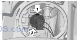
5. Close the headlamp housing with the cap. Make sure that the cap engages.
