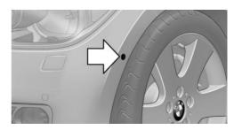
The ultrasound sensors for measuring parking spaces are located on the wheel arches.
