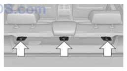
Depending on the vehicle equipment, there are two outer or three mounting points for child restraint fixing systems with a tether strap.
