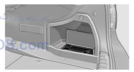
The screw-in tow fitting should always be carried in the vehicle. It can be screwed in at the front or rear of the BMW. It is in the onboard vehicle tool kit located in a storage compartment on the right side in the cargo area. Open the cover.
