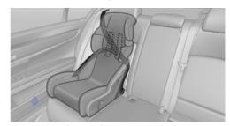
The rear safety belts and the front passenger safety belt can be locked against pulling out for mounting the child restraint fixing systems.
