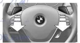
The shift paddles on the steering wheel allow you to shift gears quickly while keeping both hands on the steering wheel.
