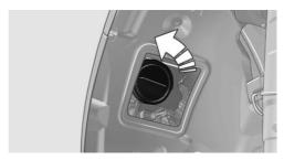
Tilt the bulb down and then up to loosen it from the holder and remove.
