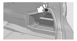
2. Pull the green knob with the fuel pump symbol. This releases the fuel filler flap.
