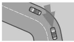
If the desired speed is too high for a curve, the speed is reduced slightly in the curve, although curves cannot be anticipated in advance. Therefore, drive into a curve at an appropriate speed.
