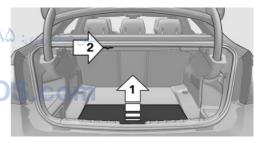
Raise the cargo floor panel, arrow 1, and latch at top, if necessary, arrow 2.
