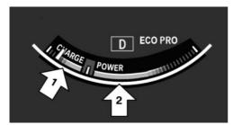
In the tachometer, a mark in the bar display indicates the current efficiency of the driving style.
