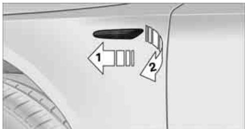
2. While simultaneously lifting the retaining tab, rotate bulb holder to the left and remove.
