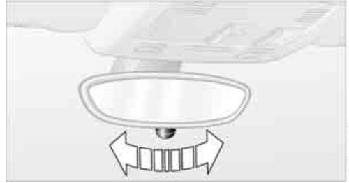
Turn the knob to reduce glare from the headlights of cars behind you when driving at night.
