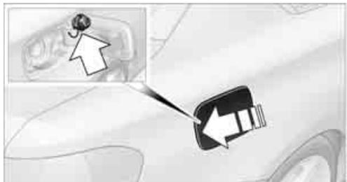
1. Open the fuel filler flap. To do so, lightly press the rear edge.
