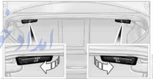
1. To release the rear seat backrest, pull the corresponding lever in the trunk.
