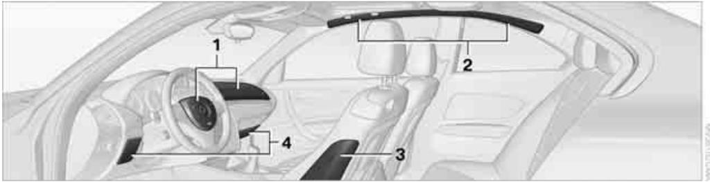
The following airbags are located under the marked covers:
