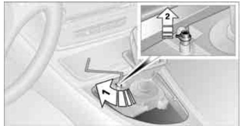
4. Insert allen wrench into the opening, arrow 1.
