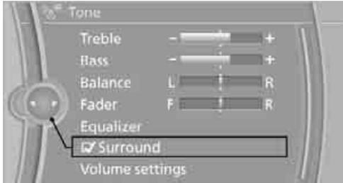
When surround is activated, multi-channel playback is simulated when playing an audio track in stereo.
