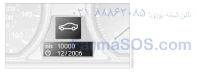
The remaining driving distance and the date of the next scheduled service are displayed briefly immediately after you start the engine or switch on the ignition.
