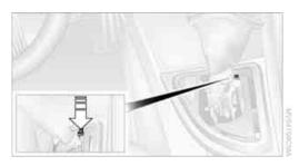
Using the screwdriver from the onboard vehicle tool kit, refer to page 227, press the red lever, see arrow, while moving the selector lever to the desired position.
