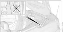
Lift out the front part of the convertible top, arrows 4, on both sides and swing it forward. At the same time keep the convertible top box cover from closing, e.g. using your shoulder.
