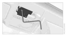
Reattach the lamp cover and reinstall the control unit.
