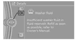
You can call up more information on the Control Display, e.g. on the cause of a malfunction and on how to respond, via Check Control, refer to page 78.
