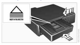
Insert the CD magazine all the way in the direction of arrow 1 and close the cover, arrow 2.
