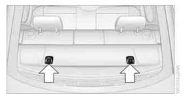
For child restraint systems with tether straps there are two additional anchors, see arrows.
