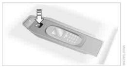
Press the button and remove the mobile phone.
