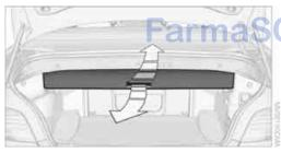
When the convertible top is closed you can enlarge the cargo area:
