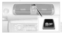
Press the button for at least 3 seconds until the indicator lamp for DSC OFF lights up and DSC OFF is displayed in the instrument panel. Dynamic Traction Control DTC and DSC have been simultaneously deactivated. Stabilizing and drive-output promoting actions are no longer executed.
