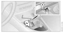
4. Insert allen wrench into the opening, arrow 1.
