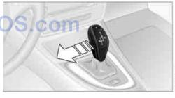
Push selector lever toward the left from the selector lever position D, the Sport program is activated. This position is recommended for a performance-oriented driving style.
