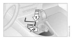
Rotate allen wrench until it reaches the stop, arrow 2. The parking lock is unlocked.
