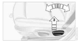
Pull lever **3** and apply your weight to the backrest or lift it off, as necessary.
