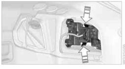
The bulbs are integrated in a single bulb holder.
