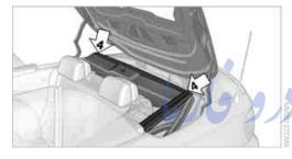
Position the rear convertible top frame upright, arrow 5, and close the convertible top box cover, arrow 6. Then lower the rear convertible top frame.
