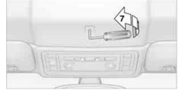
Turn the Allen wrench all the way to the left, arrow 7, until the front convertible top frame is locked to the windshield frame. The rear convertible top frame is automatically pressed down onto the convertible top box cover and is sealed tight under tension.
