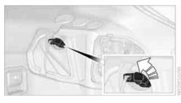
The outer brake lamp can be accessed through a single socket.
