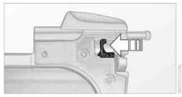
Slide the red release lever towards the middle of the wind deflector and push the two halves apart.
