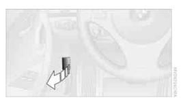
On the driver's side is an OBD socket for checking components relevant to the composition of the vehicle's emissions.
