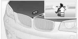
To avoid damage, make sure that the wiper arms are against the windshield before you open the engine compartment. Do not open the engine hood before the engine has cooled down; otherwise, injuries may result. ◀
