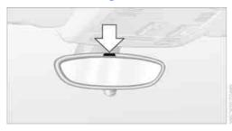
The automatic dimming feature of the interior and exterior mirrors\* is controlled by two photo cells in the interior rearview mirror. One photo cell is in the mirror frame, see arrow; the other is on the back of the mirror.
