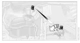
Attach one terminal clamp of the plus/+ jumper cable to the positive terminal of the battery or a starting-aid terminal of the vehicle providing assistance.
