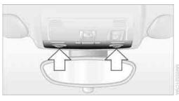
2. On both sides, use the screwdriver to press on the clip inside the opening.
