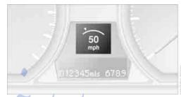
When the speed at which the vehicle is traveling is stored or when a stored speed is called up, the speed is briefly displayed in the instrument cluster.
