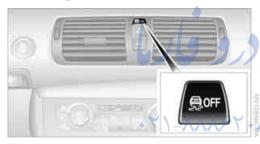
Press the button; the indicator lamp for DSC OFF lights up and TRACTION is displayed in the instrument panel.
