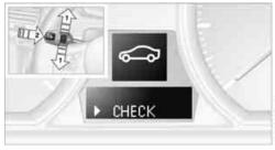
Push button 1 in the turn signal/high beam lever up or down repeatedly until the appropriate symbol appears in the display, accompanied by the words "CHECK".
