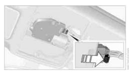
Insert the Allen wrench\* supplied with the onboard vehicle tool kit, refer to page 227, into the opening provided. Move the glass roof in the desired direction.
