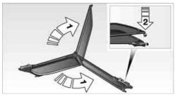
Press together the top and bottom parts of the wind deflector until the catch engages, arrow 2.
